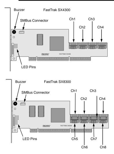
2. Attach one Serial ATA data cable to each disk drive. Then attach the other ends of the cables to the connectors on the FastTrak card (above).
